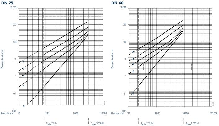
Viscosity diagrams: A = 5 mPa.s C = 50 mPa.s E = 200 mPa.s B = 25 mPa.s D = 100 mPa.s E = 500 mPa.s
