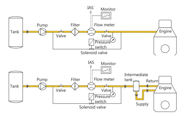
Ship classification societies require the installation of bypass pipes. The relevant regulations must be followed.
